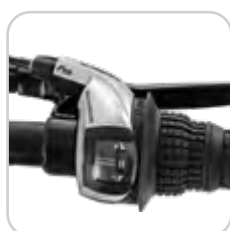
Rotating grip shifter with speed indication
