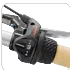
Rotating grip shifter with speed indication
