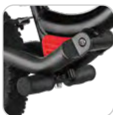
Removable PEGs made from aluminium
